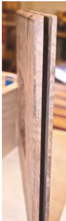
▲ Pic.3 For this project I decided to use a tiger maple board, which measured 1,524 × 125 × 20mm. I cut four pieces measuring 305mm long with 45° corners. So the grain pattern could be followed as you turn the box, I marked each of the four sides with directional arrows. Next, I cut a slot 3mm from the top of each piece, 7mm wide and 6mm deep, which would accommodate the walnut lid section. I wanted the lid to float in the slots for wood movement so no glue was used on the walnut
